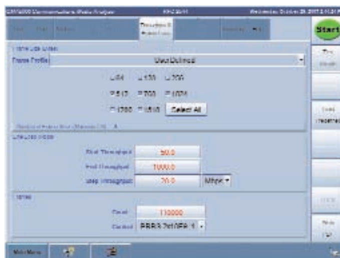
RFC 2544 details the testing requirements for deploying and commissioning high data rate networks. The CMA 5000 allows either complete control of all setup parameters or enhanced ease-of-use through automated settings.
